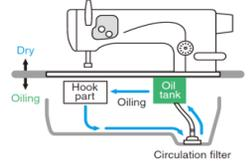
The oil dropped from the hook and its surrounding sections into the under-cover is filtered to remove dirt and dust and is then returned to the oil tank. This method saves the effort of oiling and reduces oil consumption.
