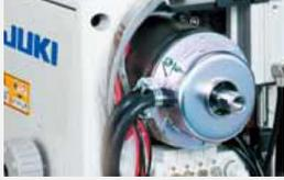
The sewing machine has adopted a high-torque direct-drive motor which is suitable for heavy-weight materials. As a result, the sewing machine is more responsive and ensures increased penetration into the material.
