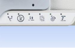
A multifunctional 6-string switch is also provided. This provides the user the ability to change the stitch length, changeover of single or double thread tension from this one switch.
