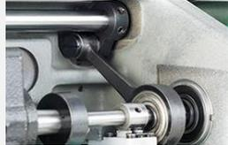
The feed driving cam is adjustable. This means the feed is changed to what is best suited to the material and thread being used.
